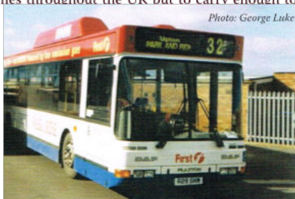
An LPG powered DAF SB220 operated by by First on the Chester Park & Ride , the gas was stored in tanks on the the roof under the two covers
