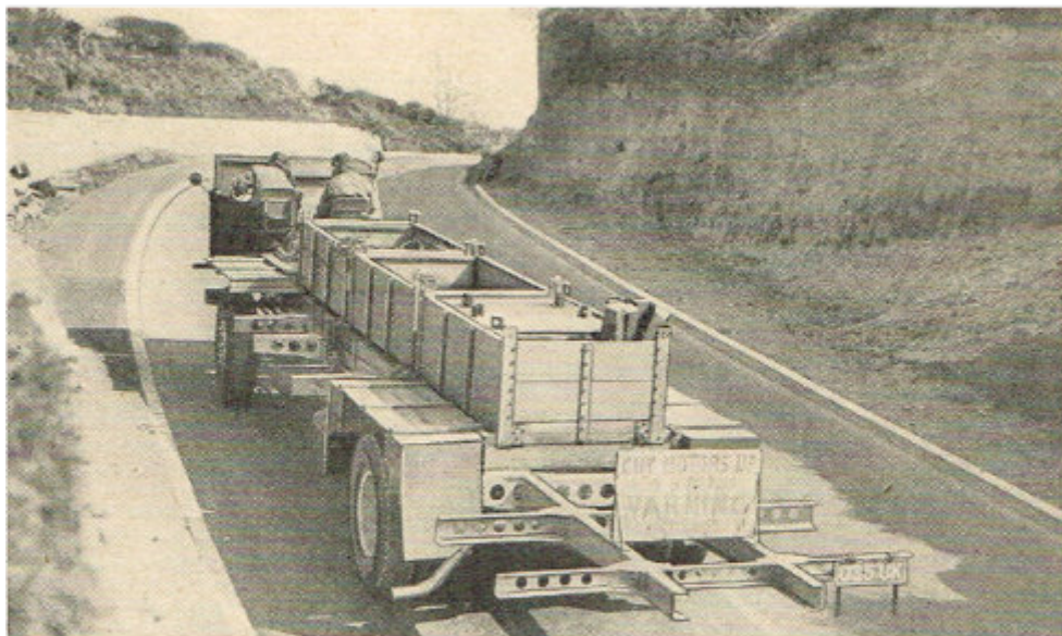
On the 1-8 section of Hermitage Hill, a smooth bottom gear restart was made at about one eighth throttle opening and without clutch slip
