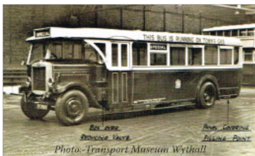
Guy Conquest BCT&OD60 in its final gas bus state. It was new in 1929 as a 25 seater normal control bus for one man operation, but was rebuilt two years later as a 32 seater half cab configuration. All the Conquests were replaced by Daimler COG5 single deckers in 1935
