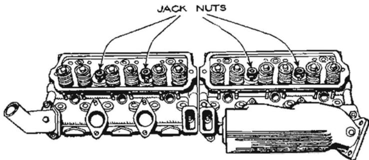
*Jack nuts for raising the cylinder heads are a feature of AEC and Leyland engines. On the AEC, the jack nuts are in the centre of the divided head. The Leyland has a one-piece head and there is a jack nut at each end.*
