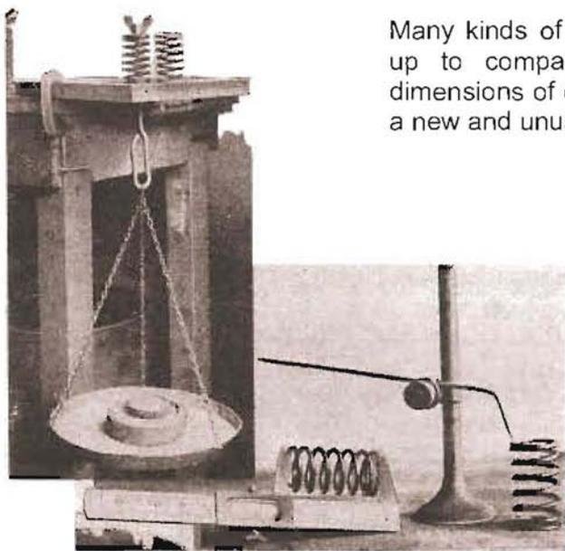
The uncompressed length is usually sufficient to warrant rejection without a compression test. Little information is available as to actual life of valve springs, and a principle followed where engines retain their own heads is to replace the springs at each complete overhaul. The method of comparison against the standard of a new spring as outlined above, works on a replacement basis of 10% below standard and is applicable to cylinder heads reconditioned under the unit replacement system.
