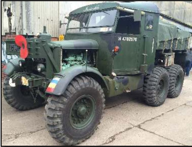
*The 6LW powered Scammell Pioneer was used for moving artillery and tank recovery*
