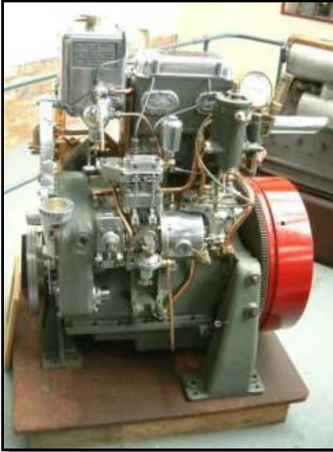
*Both the 2LW and 8LW were introduced in 1946. For marine applications the 2LW was only available with a cast iron crankcase. For other industrial applications i.e. road rollers small generator sets and other types of portable equipment then the choice of either aluminium or cast iron crankcases were offered.*
