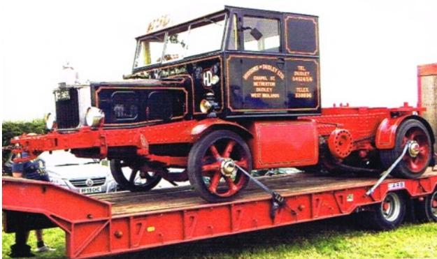
▲ One of only two built, this full restored 100 Tonner's record gross train weight was 165 tons – thanks to a 196-to-1 bottom gear.
