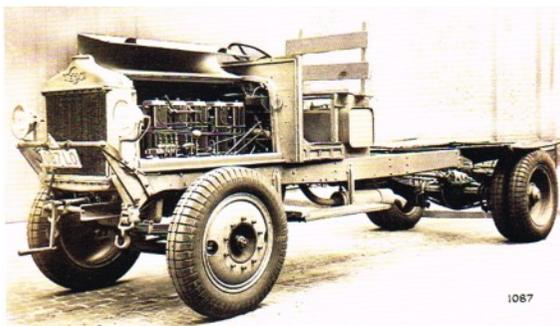
▲ Although AEC developed its own diesel engines, a Gardner five-cylinder 5L2 found its way into an AEC in 1936.
