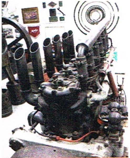
Figure 3 Exhaust side of Daimler Knight engine at the Anson Engine Museum
