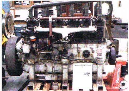
Figure 4 Inlet side of Daimler Knight engine at the Anson Engine Museum
