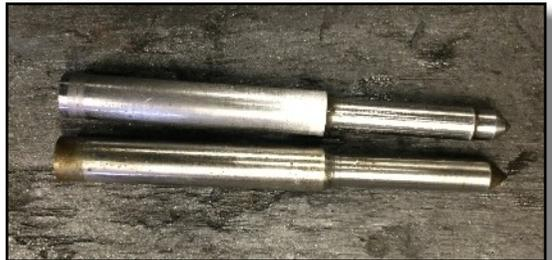
difference, the upper one being the Kromhout version. The spring pressure and lift on each sprayer was checked and if necessary reset.
