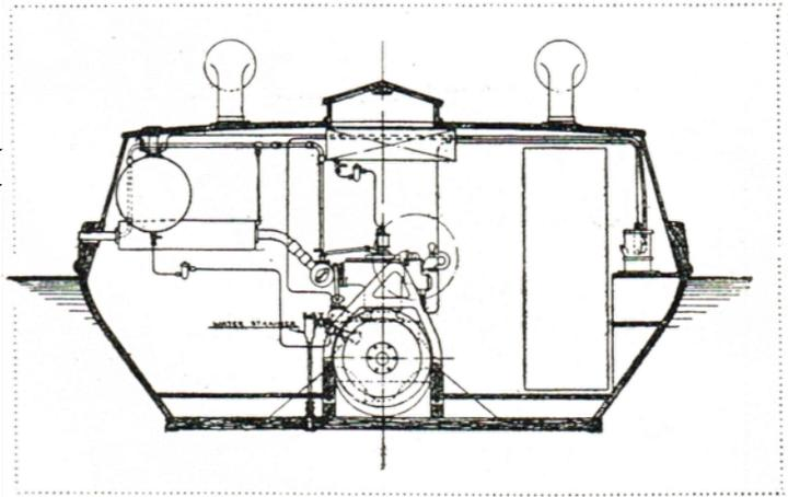
*Cross section through engine-room.*
