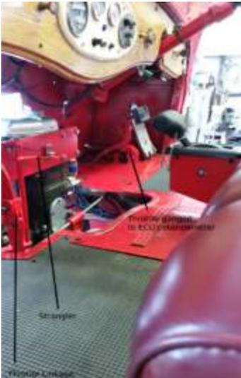
Unsure how that combination would behave on the road, the ZF was supplied with an ECU (Engine Control Unit). This is programmable from within the vehicle, so we were able to dictate under what circumstances the ZF would change gear. The shifter has the normal P, R, N, D, 1, 2, 3 configuration.
