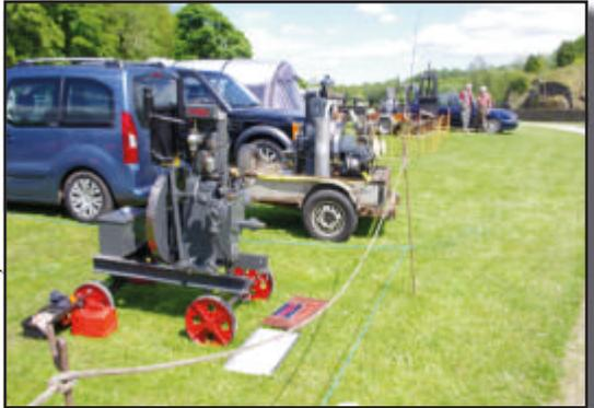
The older small stationary's, featured a No "0" and "1F" Hot tube Gas engines. Also a newly restored "1CR" spirit engine .
