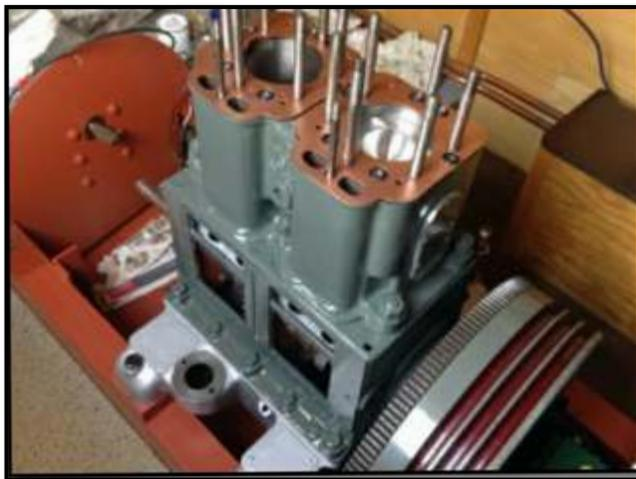
with crank / bearings/ block, conrods etc, and so started the rebuild of Enery, to my knowledge for the 3rd time in 76 years
