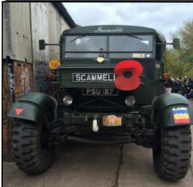
The Scammell Pioneer was developed in the late 1920s specifically for off road use. Similar vehicles were then being tested for use in the colonies where surfaced roads were scarce. The requirement matched that for military vehicles and the Army obtained a 20 ton tank recovery transporter from the Scammell Company in 1932. It was later followed by other Pioneers, gun tractors, more tank transporters and heavy breakdown tractors.
