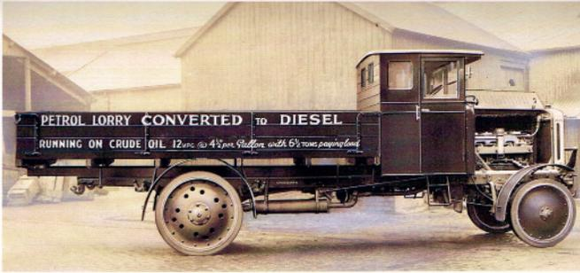
A 1930 Leyland lorry fitted with a Gardner 4L2 diesel engine.
