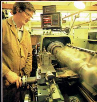
*Precision turning of a Gardner crankshaft.*
