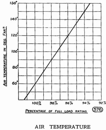
THESE have been prepared for the purpose of enabling prospective users to arrive at the approximate size of an engine required to develop a given power under any conditions of altitude and air temperature. The resulting particulars may be taken as fully on the safe side.
