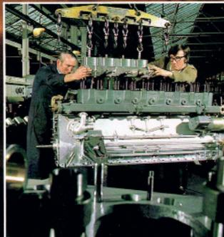
*Fitting cylinder heads to the block.*
