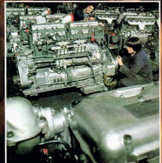
*Individual customer requirements are met at the final engine assembly.*
