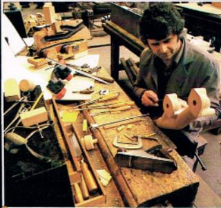
*The Gardner Pattern Shop—the origin of the engine crafted by hand in wood and resin.*
