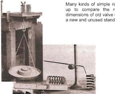
Many kinds of simple rig can be fixed up to compare the resistance and dimensions of old valve springs against a new and unused standard.
