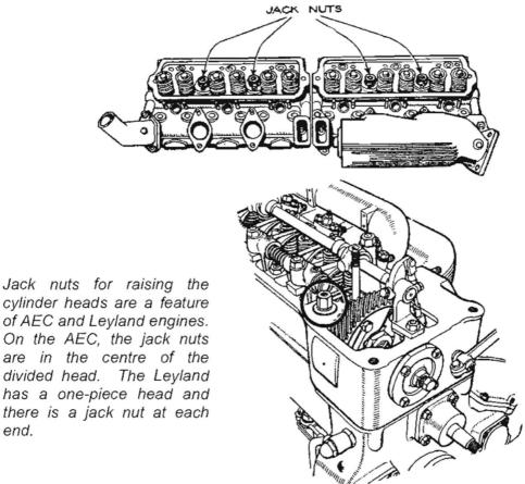
cylinder heads are a feature of AEC and Leyland engines. On the AEC, the jack nuts are in the centre of the divided head. The Levland has a one-piece head and there is a jack nut at each end
