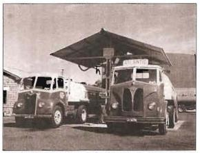
Atlantic Oils of Cape Town. Sonth Africa ran several Guy tankers. The Otter Diesel Mk.II tractor nmt is seen alongside an early Invincible Mk.1 powered by a 6LW engine, 1955.
