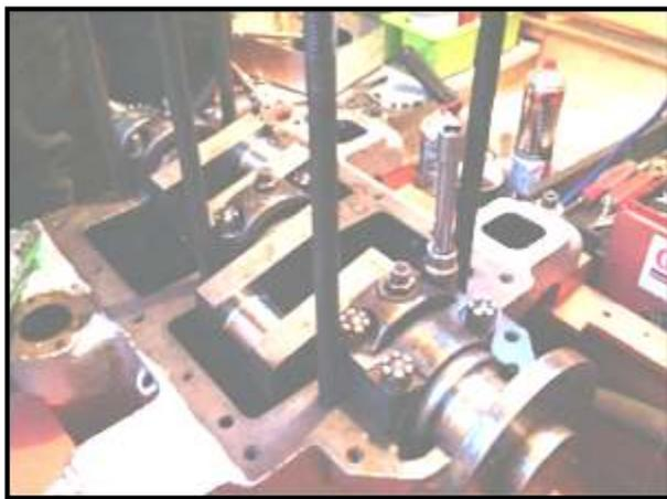
in a left hand engine, so that's why I could not cure the oil leak on the end of the crank! The cranks have a scroll to wind any stray oil back into the sump! of course mine was trying to do exactly the opposite! Also when we removed the flywheel it was fitted with the wrong sort of bolts, Charles said it was actually dangerous with all that weight spinning at 1000 revs, if it had come adrift, well it don't bear thinking
