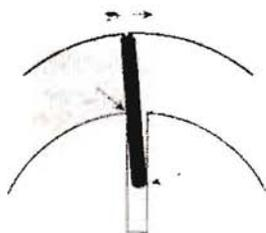
*Too much play of blades in the rotor slots results in rocking and bending, causing jamming and excessive wear at the points indicated.*
