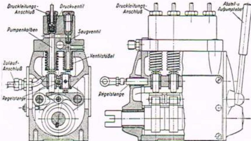
The four-cylinder Bosch plunger pump of 1923
