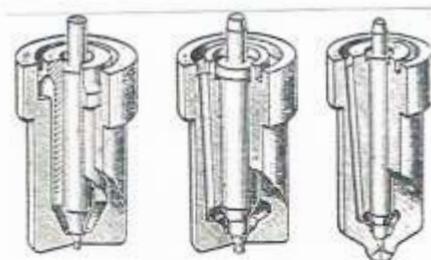
Above are seen three types of nozzle. On the left is the Acro-Lang two-part pintle, in the centre is the Bosch single-piece and on the right the Bosch multi-hole type
