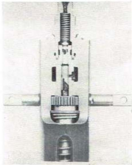
The basic Bosch pump showing the return groove in the shortened pump piston, and the radial bores in the pump cylinder to the common suction and shock chamber
