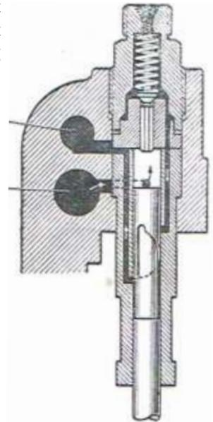
In this pump design the Bosch engineers improved upon Lang's 1926 layout by separating suction and spill chambers, therefore avoiding pressure waves in the pump suction
