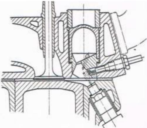
Acro air cell combustion chamber arranged in the cylinder head. Note chamfer on the piston in the region of the nozzle and the location of the heater plug. In some engines the Acro chamber was in the piston crown.
