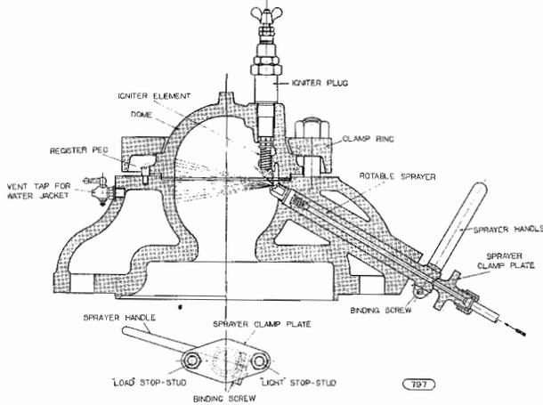
Cylinder Breech showing the Igniter Plug and Rotable Sprayer. Two positions of the Spray-form are shown : one for starting and the other (the lower one) for running at full load
